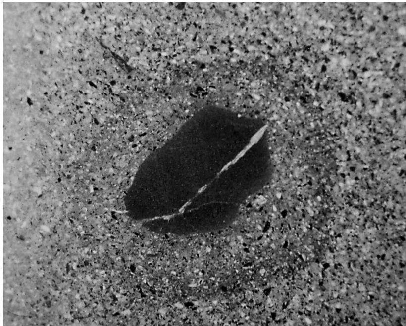
Figure 11: Photomicrograph of an un-weathered concretion inside an Omar. The calcite shale fragment at the concretions centre and the angular nature of the volcanic sand are clearly visible. The circular halo shows the extent of the original calcite concretion.
